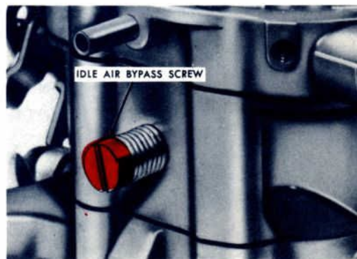
Fig. 30 Idle RPM Adjustment
