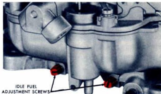
Fig. 29 Idle Fuel Mixture Adjustment
