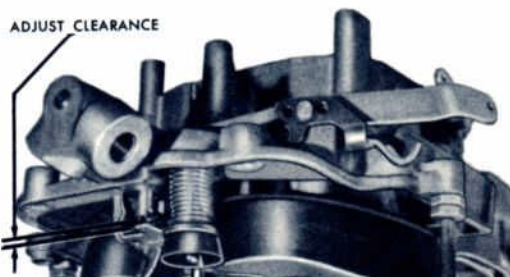
Fig. 22 Auxiliary Fuel Inlet Valve Setting
